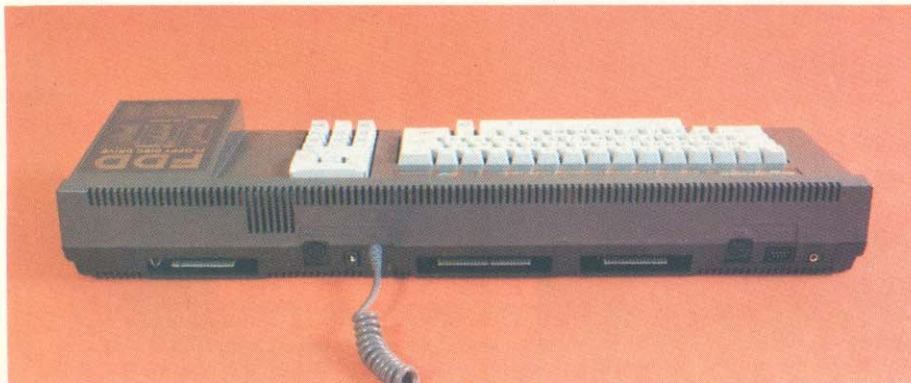
Anschlüsse (v.l.n.r.): Floppy/Monitor/5V/12V/Expansion Port/Drucker/DIN-Anschluß für Recorder/Joystick/Stereo
